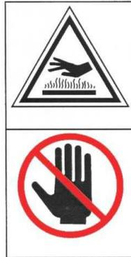
② The sign indicates the danger of burns due to contact with high temperature parts. Do not touch hot parts while the machine is operating or before having given it time to cool down after being switched off; use suitable safety equipment if necessary.
