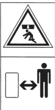
⑤ The sign indicates the hazard of crushing by unexpected movements of the accessory or bucket (if present). Keep a safe distance when the machine is operating. Always completely lower the bucket and accessory before leaving the machine unsupervised.
