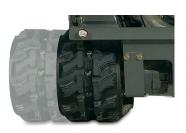
**ADJUSTABLE TRACKS** Hydraulically adjust the track width for added stability and traction, and to fit through narrow doorways and gates for interior or exterior projects
